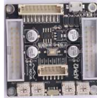
Figure 2 2 x In, 3 x Out Audio Digital Signal Processor Evaluation Version - APM2 AA-AP23122
