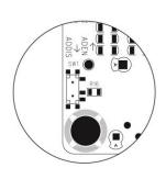
**SW1** on the backboard can be used to turn off the Signal Detection Function. When the switch is turned to ADDIS, the signal detection fuction will be turned off. Take the silkscreen on board for reference.
