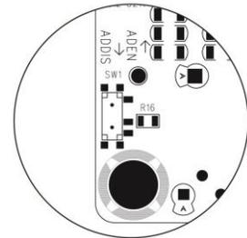
SW1 on the backboard can be used to turn off the Signal Detection Function. When the switch is turned to ADDIS, the signal detection function will be turned off. Take the silkscreen on board for reference.
